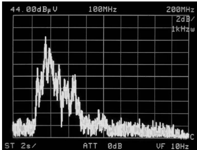
Figure 6, Background Spectrum when turned Off - Model 124A
